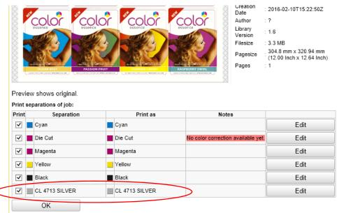
Process the file and the metallic ink will be printed for the CL 4713 SILVER separation underneath the CMYK separations, producing the Color-Logic special effects.
