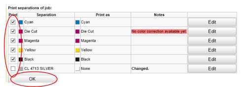
Process and print the file. The CMYK artwork will be printed on top of the white ink and in register with the previous print, allowing the reflection from the metallized substrate.
