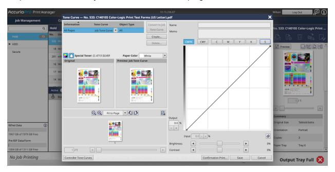
Step 4: Invert the tone curve by moving end points of tone curve to opposite corners (should resemble the below image).
