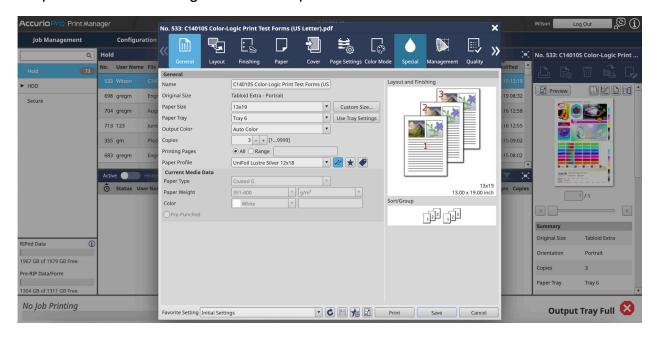
Step 8: You can utilize "Special Toner Density" in order to reduce white toner density. This is also the location where we can re-map and define the CL 4714 SILVER spot color to the white channel for the AccurioPress C14010S and C12010S.
