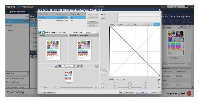
Step 6: If some elements are missing, it is likely the white plate is too opaque. To reduce the white density/gradation, first highlight job and then select Job Settings...
